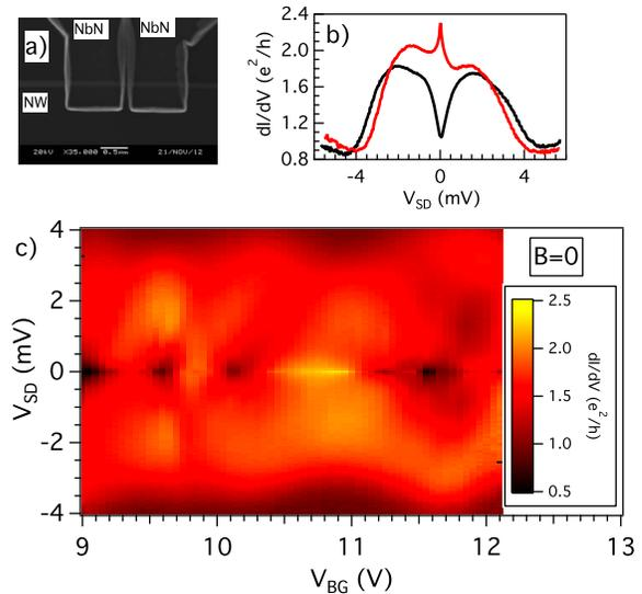
FIG. 1: (a) SEM image of NbN leads on InAs nanowire (NW). The white feature at the edges of the NbN leads is PMMA residue from the ion milling. (b) Transport at  $B = 0$  for  $V_{BG} = 10.1$  V (black) and 10.9 V (red). (c) Stability diagram at  $B = 0$  for region of interest.
