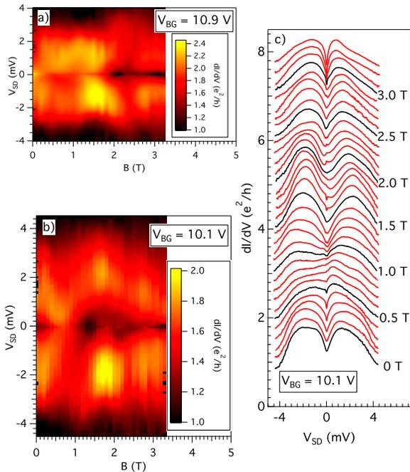
FIG. 2: (a) and (b) Conductance traces vs magnetic field for two different densities. (c) Individual traces for  $V_{BG} = 10.1$  V, each trace differing by 0.1 T. Adjacent curves are offset for clarity.
