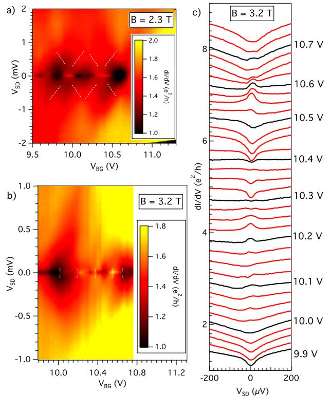
FIG. 4: Stability diagram at (a)  $B = 2.3$  T and (b)  $B = 3.2$  T. In (a), dashed white lines show location of resonant levels. In (b), dashed white lines delineate individual periods of ZBA oscillations. (c) Individual traces for  $B = 3.2$  T in steps of  $\Delta V_{BG} = 0.025$ , with adjacent curves offset for clarity.
