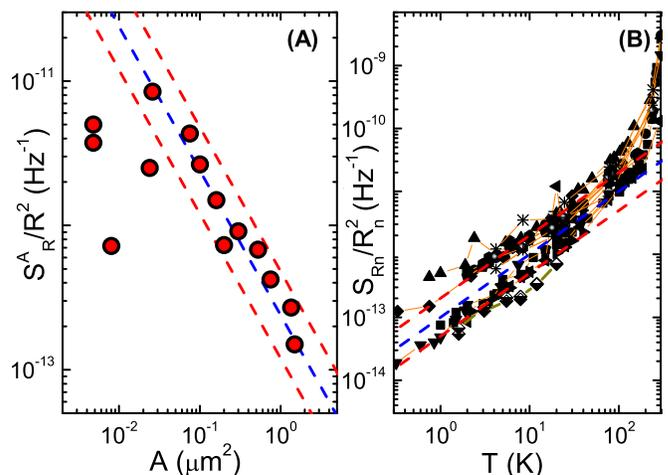
FIG. 3. (A) Area dependence of the  $S_{R_n}/R_n^2$  ( $f = 1 \text{ Hz}$ ) in unshunted junctions at  $T = 2 \text{ K}$ . Note the deviation from the linear scaling at  $A \sim 0.04 \mu\text{m}^2$ . (B) Temperature dependence of  $S_{R_n}/R_n^2$  in unshunted junctions. The noise value is quoted at  $f = 1 \text{ Hz}$  and is area normalized to  $A = 1 \mu\text{m}^2$ . The dashed lines depict the average noise value as well as its upper and lower bounds (see text).
