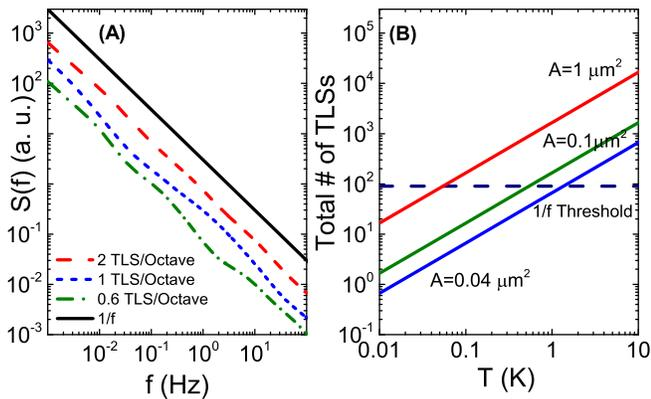
FIG. 4. (A) Simulated noise resulting from averaging over different number of TLSs per frequency octave. (B) Amount of fluctuators extracted from measured  $1/f$  noise as function of temperature for several junction sizes. Dashed line shows statistical threshold for featureless  $1/f$  noise.
