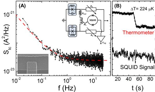
FIG. 1. (A) Critical current power spectrum measured at  $T = 315$  mK, and  $I_b/I_c = 1.05$ . The dashed line is a fit to  $1/f +$  a white noise component. Top inset: Schematic representation of the bridge-SQUID potentiometry circuit. Bottom inset: SEM image of the Al/AlO<sub>x</sub>/Al junctions. (B) Time traces of the sample temperature and the SQUID signal, monitored across a small temperature perturbation at  $T = 315$  mK for  $I_b/I_c = 1.05$ .
