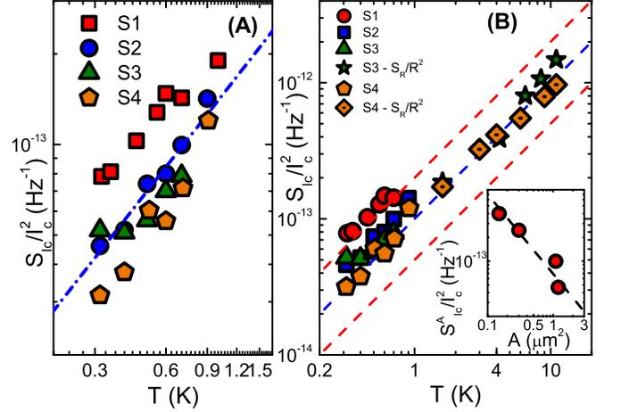
FIG. 2. Temperature dependence  $S_{I_c}/I_c^2$  (A) and  $S_{I_c}/I_c^2$  with  $S_{R_n}/R_n^2$  (B) at  $f = 1$  Hz in several sets of devices. The noise values are area normalized to  $A = 1 \mu\text{m}^2$ . The dashed line shows linear T dependence (see text). Inset: Critical current noise (not area normalized),  $S_{I_c}^A/I_c^2$ , at  $T = 500$  mK as a function of junction area. The dashed line depicts  $1/A$  dependence.
